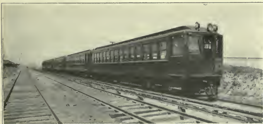
FIG. 535. MULTIPLE-UNIT TRAINS. Multiple-Unit Train for 600-Volt Direct Current Third Rail Operation, Long Island Railroad.
